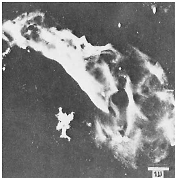
Fig. 12. Electron micrograph of cross section of DMDHEU-treated cotton of 0.71% nitrogen immersed in 0.5M cuene for \frac{1}{2} hr. Note partial dissolution of the cross section and distortion in the morphology due to swelling as compared to the cellulase-treated cross section in Fig. 11.
